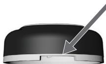
**2** Grasp the top of the End Cap and twist slightly clockwise until the pins line up with the vertical slots on the body of the Qtube.
