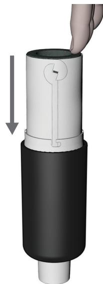
**8** To reassemble, ensure that the O-ring is seated in the groove at the bottom of the end cap, align the pins on the end-cap, and push downwards, and twist slightly counter-clockwise until the pins return to the locked position. Finally, replace the retaining clip by firmly pressing straight down until it “clicks” into place.
