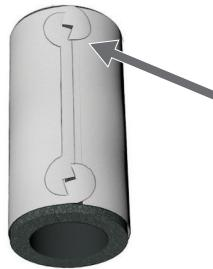
**6** Take the new inner foam baffle material and place this on top of the plastic sleeve liner. Roll the foam material so that the edges of the plastic sleeve liner meet and the tabs are adjacent to each other. Once the tabs are aligned, slip one of the tabs past the other such that they interlock.
